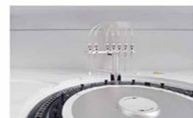
Washing Probe Independent 7-step washing system.
