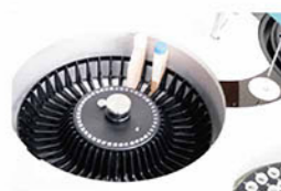
Reagent Tray 2~8°C cooling for 24 hours.
