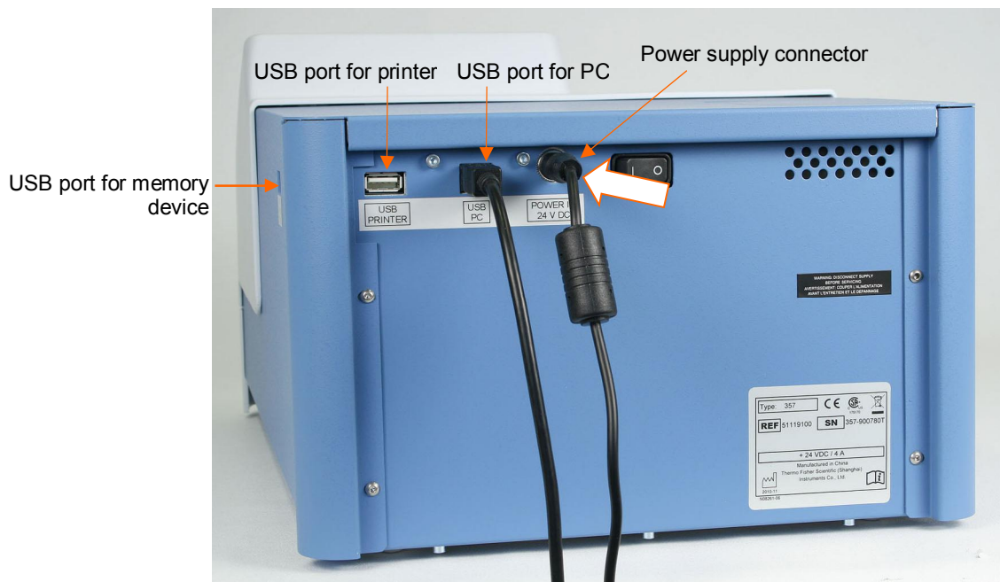
Figure 9. Connecting the power supply cable
