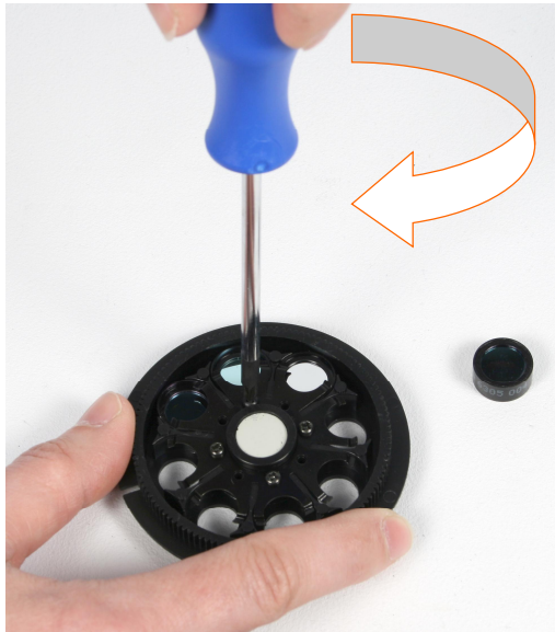
Figure 20. Removing the spring position holding screws
