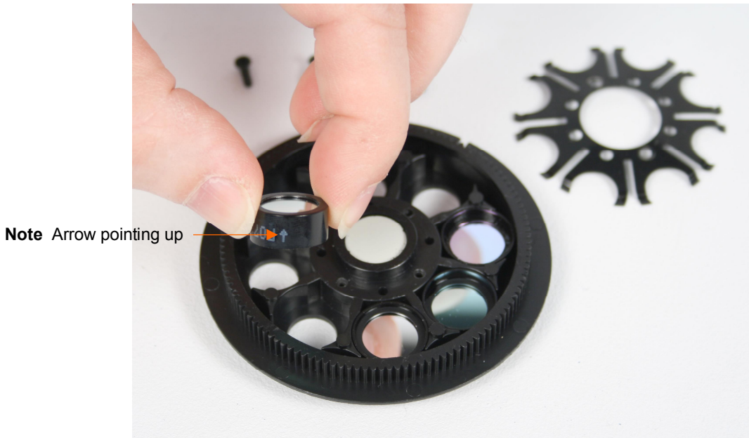
Figure 23. Inserting a filter into the next free position in the filter wheel
