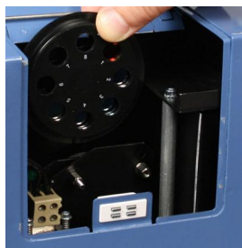
Figure 8. Placing the Multiskan FC filter wheel into the filter slot
