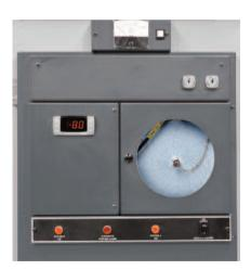
**Control system** features a digital temperature display, 6" circular chart recorder, independent refrigeration controls, a keyed master switch and indicator lights for all control and operational functions.
