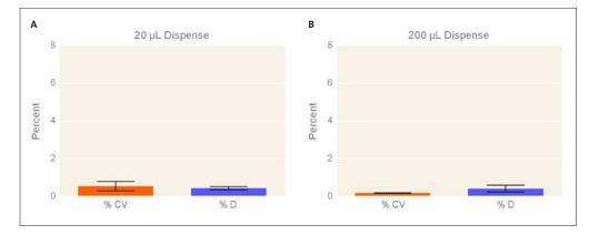
Figure 1. Analysis of EV-200-R tip with aqueous dispense. The precision (assessed by % CV) and accuracy (assessed by % D) of Axygen EV-200-R tips dispensing (A) 20  $\mu$ L and (B) 200  $\mu$ L volumes using the Tecan Freedom EVO liquid handling workstation were determined using the Artel MVS<sup>®</sup> system. The % CV and % D were below 1% for both the 20  $\mu$ L and 200  $\mu$ L dispenses, n = 288.
