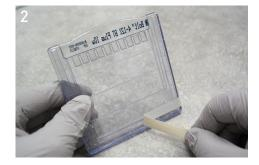
**2.** Remove the comb, and peel away the tape at the bottom of the gel cassette.
