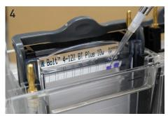
**4.** Make sure the wells are completely filled with 1X buffer.
