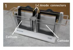
Snap the electrophoresis tank into the base, and place the cassette clamp(s) into the chamber(s) with the anode connector(s) (+) aligned to the center.
