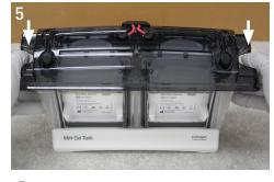
**5.** Make sure the power supply is **off**. Place the lid on the tank and plug the electrode cords into the power supply. Turn the power supply on to begin transfer.
