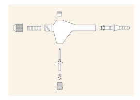
To clean, immerse the pieces in mild laboratory detergent, but do not use abrasives, as a roughened surface may affect the smooth operation of the control valve. When working with salt-rich solutions, rinse out the aspirator handpiece with distilled water after use to avoid build-up of dried deposits.
