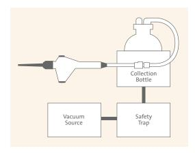
The aspirator is designed for use with a vacuum pump or an in-house vacuum system and a suitable collection vessel.
