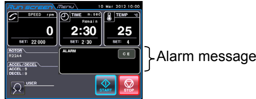
Fig.4-1 Displaying an alarm message
