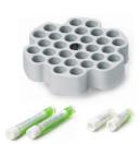
To ensure cell freezing rate consistency and uniform results when using Corning CoolCell containers, insert a CoolCell Filler Vial into the empty wells when freezing less than a full load. It is suitable for repeated use and compatible with CoolCell LX, CoolCell FTS30, and CoolCell 5 mL LX containers.
