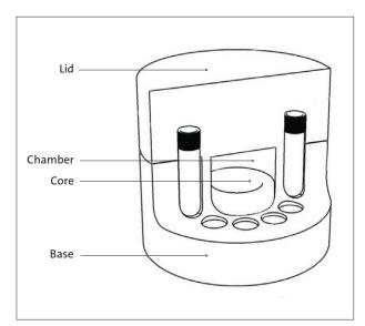
Corning CoolCell LX uses a combination of uniform-density cross-linked polyethylene foam, a solid state core, and radial vial symmetry to create freezing profiles that are consistent and reproducible. The low heat content also ensures that CoolCell LX containers will rapidly return to room temperature when removed from the freezer.
