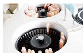
Reagent Tray 2~8°C cooling for 24 hours.
