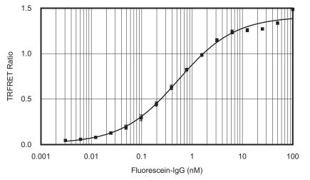
Figure 3—Titration of Fluorescein-Mouse IgG into Tb-Anti-Mouse antibody on the Tecan Ultra.
