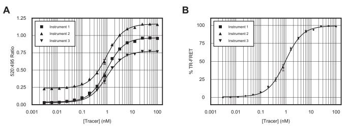
Figure 4—Assay window variability due to instrument type does not affect the resulting data and upon normalization, the above three curves are identical.
