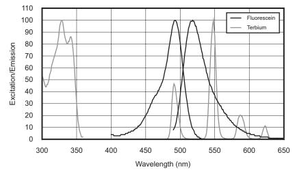
Figure 1—Excitation and Emission spectra of fluorescein and terbium.
