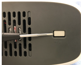
Figure 3 USB port dust cover (Rear view of PowerEase™ Touch 350W Power Supply)
