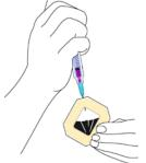
**Figure 7.** Add air to the cassette containing the sample.
