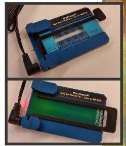
MiniTherm Slide Warmer with two-armed keeper and Temperature Validation Slide
