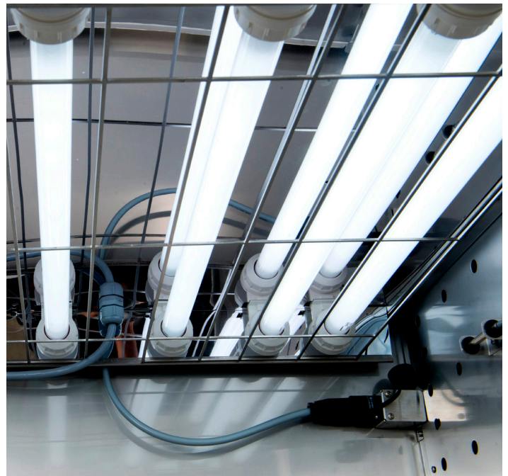
Interior of Forma Vertical Light Chamber with animal hatching light modules installed.
