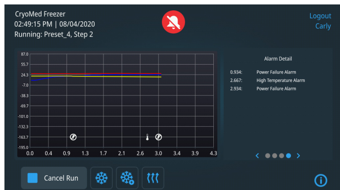
Figure 85. Alarm Detail Screen
