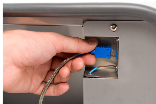
Figure 4. Sample Thermocouple Connection
