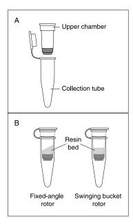
Figure 2. Spin filter. (A) An empty filter showing the separate parts. (B) Appearance of the resin bed after centrifugation in a fixed-angle rotor or swinging bucket rotor.
