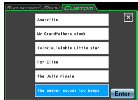
Fig. 3-4-5 (2) Stop signal setting screen
