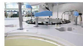
Mixer Probe Dual mixer, auto frequency adjustment
