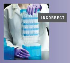
While grasping lower portion of the blister sleeve, lift sleeve up off rack and transfer entire sleeve to an empty rack. Make sure to align sleeve knockouts with latch and rear lid posts.
