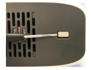
Figure 3 USB port dust cover (Rear view of PowerEase<sup>™</sup> Touch 120W Power Supply) The USB port is shipped with a plastic dust cover for protection during shipment. This cover must be removed prior to port use. Remove by gently prying off with a small flat blade screwdriver.
