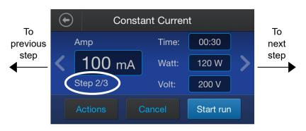
Figure 11 Method step number location
