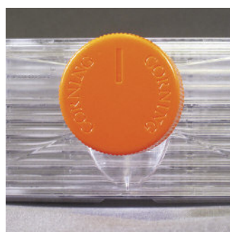
Figure 1. Venting position to be used when pre-warming the HYPERFlask and HYPERFlask M vessels when the vessel is empty or contains low volumes of liquid for prolonged periods of time (greater than 60 minutes).
