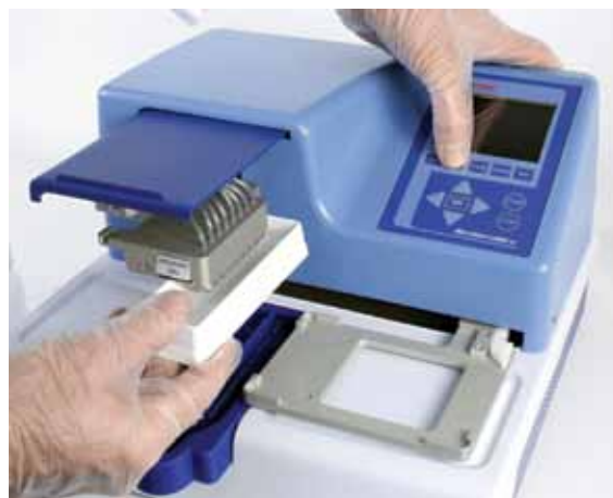
Cleaning the tubings using a reagent basin.
