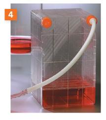
Once filling is complete, turn the CellSTACK chamber 90° so that the filling and venting ports are up (as shown). It is normal for the medium level in the bottom chamber section to be slightly higher. Replace the filling cap with the original vented cap and the vented cap with a venting filter or solid cap (Cat. No. 3969).
