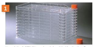
Unpack the CellSTACK vessel, and place it inside a laminar flow hood or clean room environment to carry out aseptic connections.
