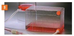
Ensure the dispensing vessel is elevated above the CellSTACK vessel. Connect the MPC from the filling cap to the MPC from the filling vessel. Open the clamp to start filling. Medium will level out between layers during filling.
