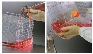
To fill the CellSTACK vessel by hand, tilt the vessel slightly toward the filling port. Smaller CellSTACK vessels can also be emptied by hand by carefully pouring from the filling port into a sterile collection vessel.
