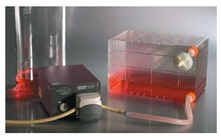
If using a peristaltic pump for filling and emptying, it is recommended to replace the vent cap with a venting filter to prevent potential shearing, media foaming, or cracking of the vessel.
