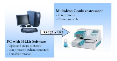
Figure 1-1. Operation principle
