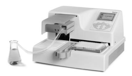
Figure 1-2. Multidrop Combi microplate dispenser
