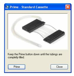
2. Click **Prime** and keep the button pressed down until the tubings are filled. The instrument primes the dispensing system.
