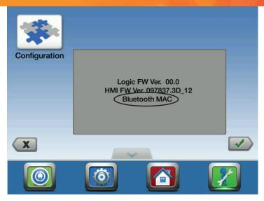
Refer to the VersaCool bath circulator's **Configuration** display to identify its **Bluetooth Mac** address, as seen on the mobile app list.
