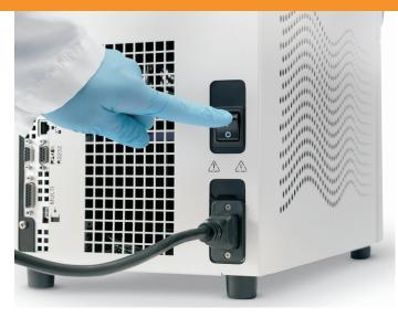
The Bluetooth connection is enabled as soon as the power cord is connected and the circuit protector located on the rear of the bath is placed to the  ${\bf I}$  position.
