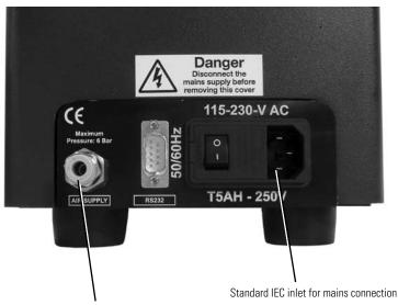
Standard ¼ BSP to 6mm pneumatic connection
