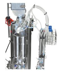
Figure 9. Cable/tubing management system.
