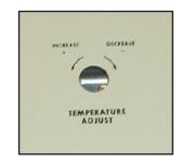
The temperature of the process fluid to your application is adjusted by turning the recessed
