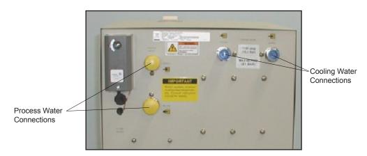
Flexible tubing, if used, should be of heavy wall or reinforced construction. All tubing should be rate to withstand 80 psi at +35°C. Make sure all tubing connections are securely clamped. Avoid running tubing near radiators, hot water pipes, etc. If substantial lengths of tubing are necessary, insulation may be required to prevent loss of cooling capacity.
