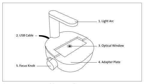
Figure 1. Instrument overview of the Corning Cell Counter.
