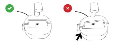
Figure 16. Correct adapter plate placement
