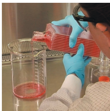
Figure 6. This initial pouring position allows medium to flow over the air dam and reduces foaming.
