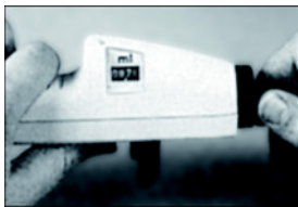
Fig. 4-5: Setting the volume
