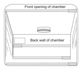
Figure 1-16. Four Rods Installed in Chamber
