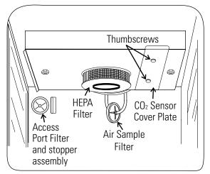
Figure 1-17. Filter and Plate
