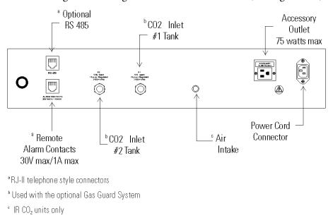
Figure 6-5. Unit Back Connections
