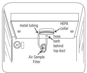
Figure 1-18. Air Sample Filter Installation
