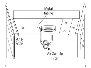
Figure 5-8. Connect to Metal Tubing
