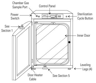
Figure 1-1. Steri-Cycle Components
