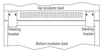
Figure 1-8. Installed Brackets on Back of Unit
