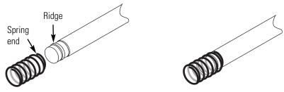
Figure 1-14. Spring Assemble to Rod
