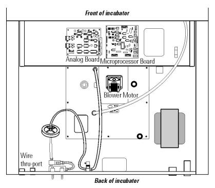
Figure 6-3. Analog Output Board Location
