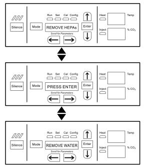
Figure 5-14. Displays with IR Sensor Removed
