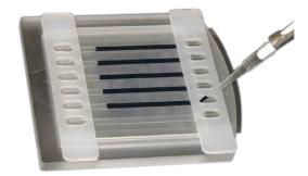
**Note:** You do not need to fill the remaining wells with sample buffer if you are not using all sample wells. You may run 1–6 IPG strips per ZOOM<sup>®</sup> IPGRunner<sup>™</sup> Cassette. Leave unused wells empty.
