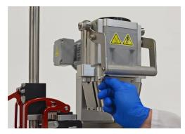
Figure 3.8. Pushing button on hub cover.
