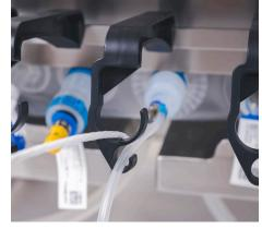
Figure 3.59. RTD placed in a probe clip.
