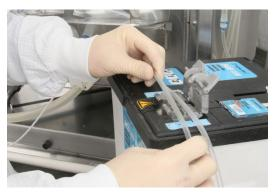
Figure 3.82. Tubing welder.
