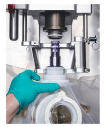
Figure 3.40. Aligning bearing hub with the bearing.
