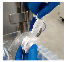
Figure 3.69. Pulling the tabs to remove the paper membranes.
