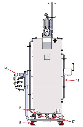
Figure 4.4. Back view of 500 L DynaDrive S.U.B. (with optional E-Box).
