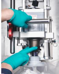
Figure 3.41. Pulling down on BPC lift lever and locking mechanism.
