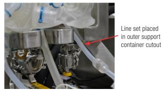
Figure 3.22. All line sets placed in proper cutouts.
