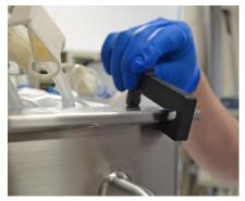
Figure 3.15. Placing the black top tab holders on the top front of tank.
