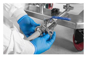
Figure 2.3. Attaching water jacket port using tri-clamp.
