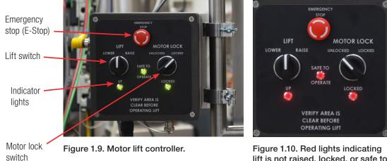
lift is not raised, locked, or safe to operate.
