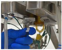
Figure 3.19. Pulling down on the white pin.
