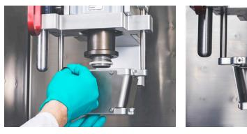
Figure 3.37. Pushing button on hub cover.
