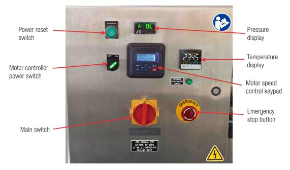
Figure 4.9. Front view of the E-Box for 50 and 500 L DynaDrive S.U.B.s.
