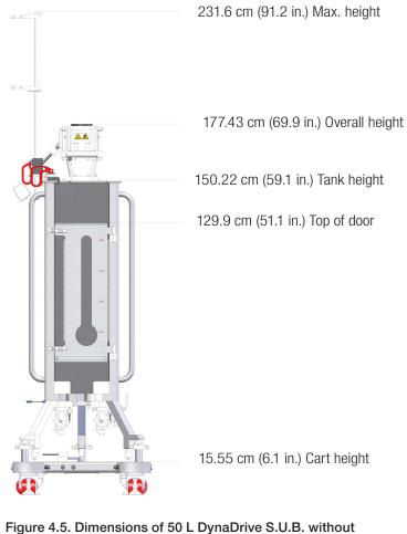
Figure 4.5. Dimensions of 50 L DynaDrive S.U.B. without optional E-Box (front view).
