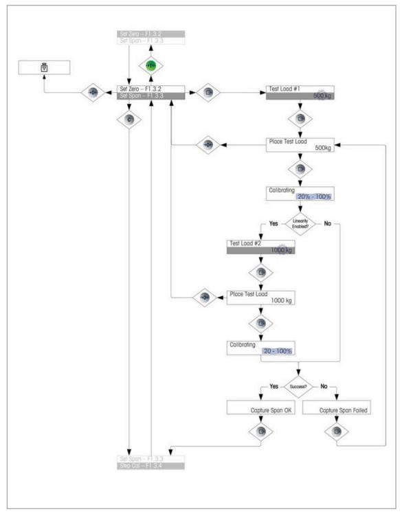
Figure B.1. Span calibration.
