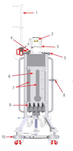
Figure 4.1. Front view of 50 L DynaDrive S.U.B. (without optional E-Box).
