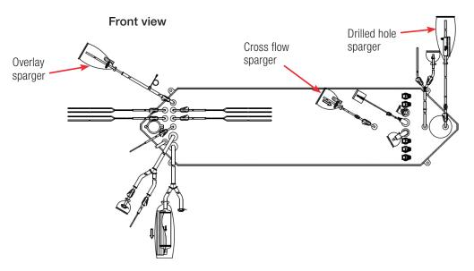
Figure 3.77. 500 L DynaDrive S.U.B. BPC spargers.
