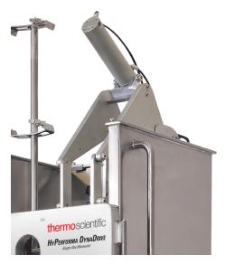
Figure 1.8. Pneumatic motor lift.
