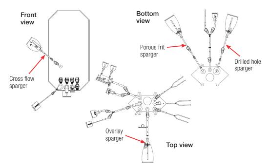
Figure 3.76. 50 L DynaDrive S.U.B. BPC spargers.
