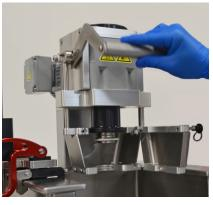
Figure 3.10. Raising BPC lift mechanism lever.
