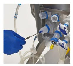
Figure 3.28. Inserting the RTD.
