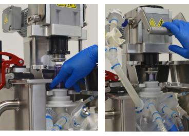
Figure 3.11. Aligning bearing hub with the bearing.
