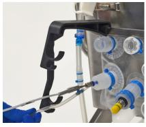
Figure 1.15. Double probe clip.
