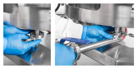
Figure 2.4. Removing the tri-clamp and attaching the fitting.
