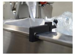
Figure 3.56. Placing the black top tab holders on the top front of tank.
