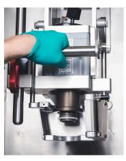
Figure 3.39. Raising BPC lift mechanism lever.
