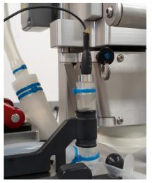
Figure 3.78. 50 L Foam probe in foam probe holder.
