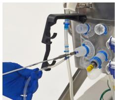
Figure 3.29. RTD placed in a double probe clip.
