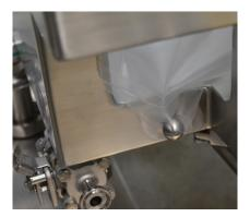
Figure 3.51. BPC bottom hanging tab attached to bottom pin.
