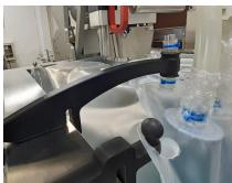
Figure 1.18. 500 L foam probe holder.
