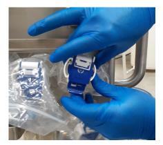
Figure 3.65. Removing plastic covering from the connector.
