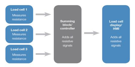
Figure 1.13. Load cell system overview.
