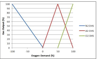
Graph 3.1. Example of a drilled hole sparger DO control strategy for DynaDrive S.U.B. systems.
