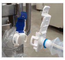
Figure 3.67. Aligning the connectors.
