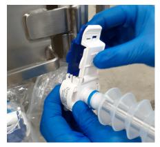
Figure 3.68. Squeezing the two connectors together.
