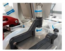
Figure 1.17. 50 L foam probe holder.
