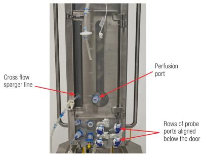
Figure 3.24. Door shut, with lines and ports aligned in cutouts.
