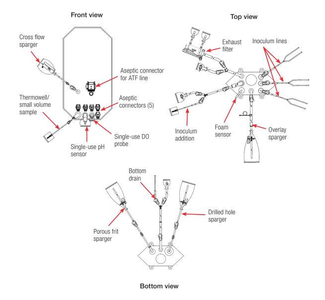
Figure 4.11. Front, top, and bottom views of 50 L DynaDrive S.U.B. BPC with ATF.
