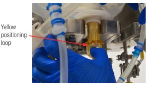
Figure 3.18. Yellow positioning loop aligned with the center cutout.
