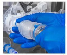
Figure 3.71. Collapsed bellows.
