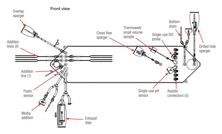
Figure 4.13. Front, top, and bottom views of 500 L DynaDrive S.U.B. BPC.
