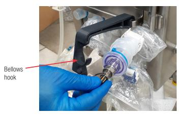
Figure 3.72. Lifting the probe before setting it into the bellows hook.
