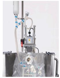
Figure 3.48. Pneumatic motor lift in lowest position.
