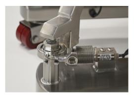
Figure 1.14. Load cell location.
