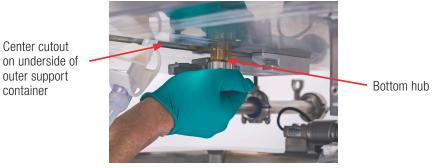
Figure 3.43. Sliding the bottom hub into place in the front center cutout.
