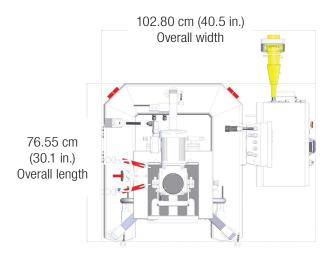
Figure 4.6. Dimensions of 50 L DynaDrive S.U.B. with optional E-Box (top view).
