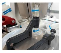
Figure 3.30. Foam probe in foam probe holder.
