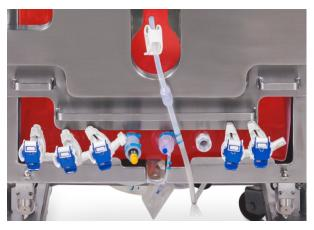
Figure 3.53. Probe port row aligned underneath the closed door (BPC shown filled).
