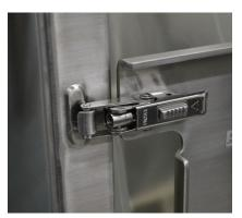
Figure 3.27. Door latch secured.
