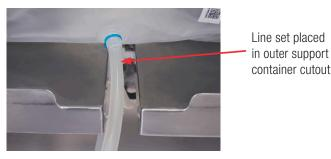
Figure 3.50. Line sets placed in bottom cutout.
