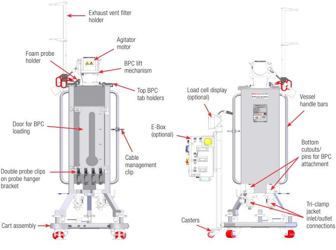
Figure 1.2. Front view of 50 L DynaDrive S.U.B. (without optional E-Box).
