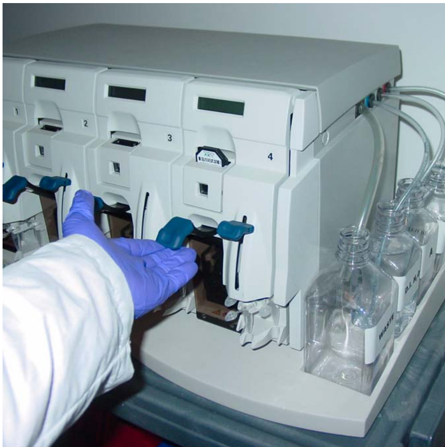
Figure 2.6 Flip the cartridge lever up to engage the cartridge septa needles into the septa.
