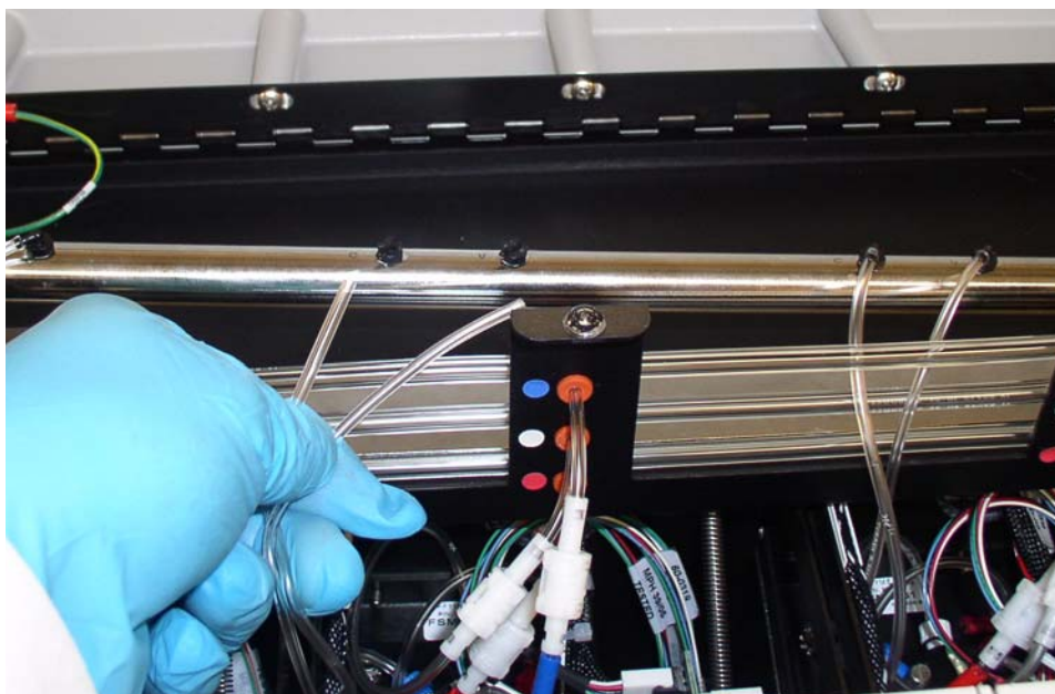
Figure A.8 Reconnect the clear, waste line tubes from the module to the drain tube.
