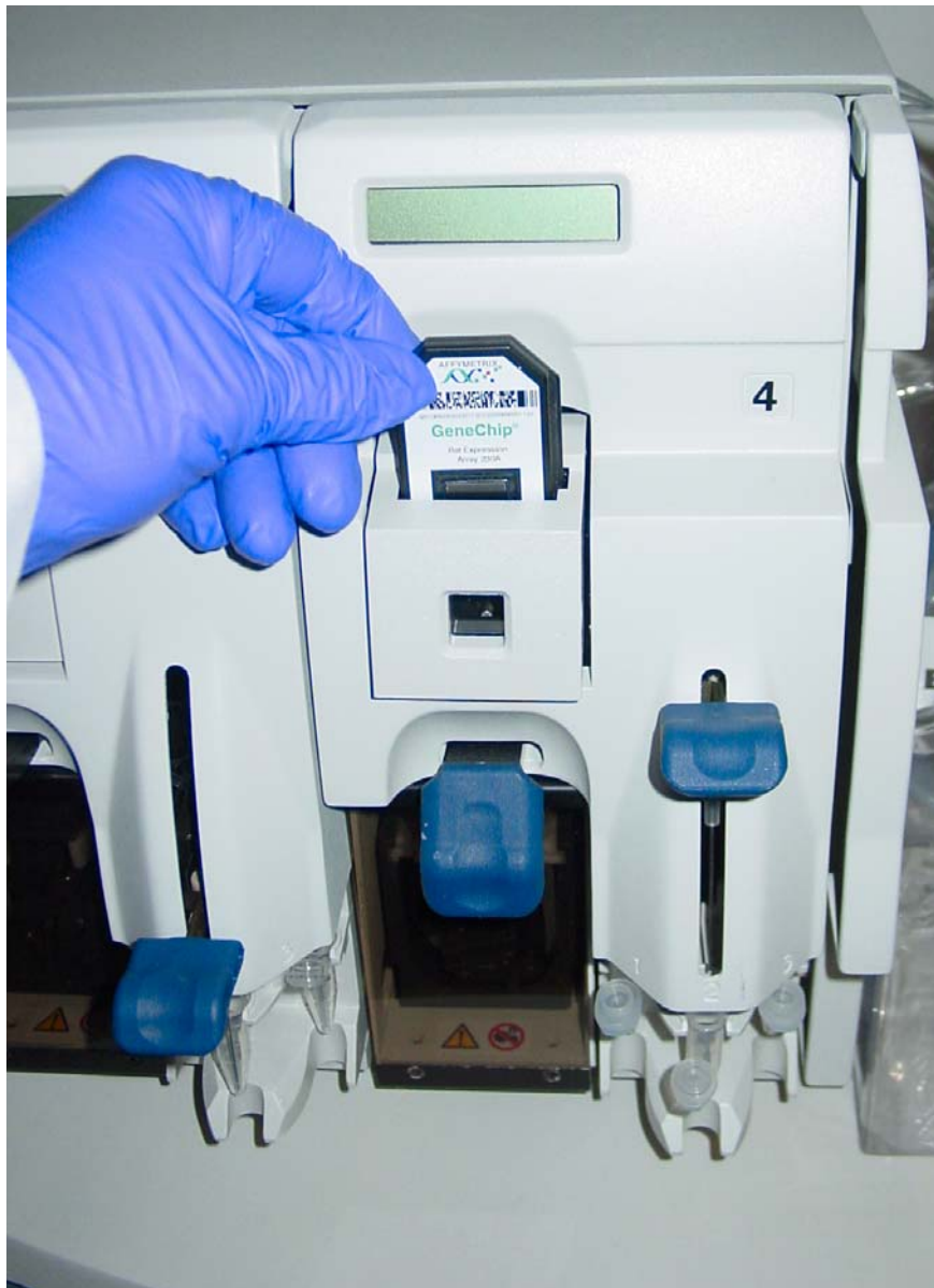
Figure 2.5 Inserting the cartridge into the cartridge holder - note orientation and probe array label
