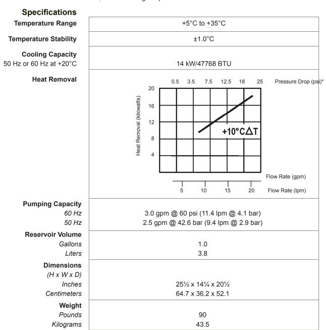
Specifications obtained using water as the recirculating fluid and using water as a coolant on secondary loop, at nominal operating voltage. Other fluids, process temperatures, ambient temperatures, altitude, or operating voltages will affect performance. Specifications subject to change. Heat load removal is based on a 10°C difference between the temperature of the cooling water supply (house water) and the cooling fluid as it leaves the System.
