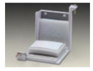
The blot module can easily be inserted in the lower buffer chamber of the mini-cell.
