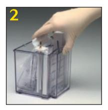
Lock the gel tension wedge in place, load samples, and fill the buffer chambers with the appropriate running buffers.
