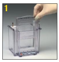
Drop buffer core into the lower buffer chamber of the XCell <code>SureLock</code>\* Mini-Cell, insert one mini-gel in front of the buffer core and a second mini-gel or the buffer dam behind the buffer core.
