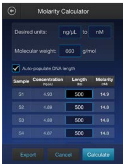
Figure 4. Integrated post-results molarity and normalization calculators. Use the molarity calculator to convert values to molarity based on nucleic acid length. Use the normalization calculator to determine how to dilute the samples to the same concentration.
