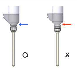
10. Press the push-button on the Neon<sup>™</sup> Pipette to the first stop and immerse the Neon<sup>™</sup> Tip into the cell-DNA/siRNA mixture. Slowly release the push-button on the pipette to aspirate the cell-DNA/siRNA mixture into the Neon<sup>™</sup> Tip.
