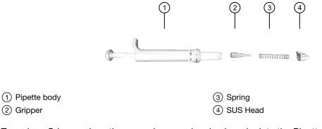
4. To replace Gripper, place the new gripper and spring in order into the Pipette body.
