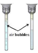
11. Insert the Neon<sup>™</sup> Pipette with the sample vertically into the Neon<sup>™</sup> Tube placed in the Neon<sup>™</sup> Pipette Station until you hear a click sound. Ensure that the pipette projection is inserted into the groove of the pipette station.
