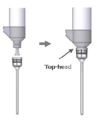
**9.** Gently release the push-button, continuing to apply a downward pressure on the pipette, ensuring that the tip is sealed onto the pipette without any gaps.
