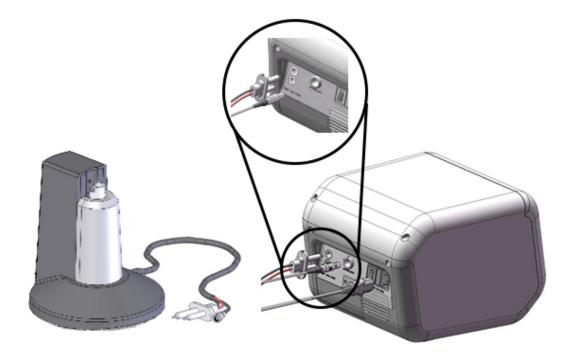
Be sure to align the ridge indicated by a white arrow on the sensor connector on the Neon<sup>TM</sup> Pipette Station with a groove indicated by a white dot on the sensor port of the Neon<sup>TM</sup> device (see figure for details).
