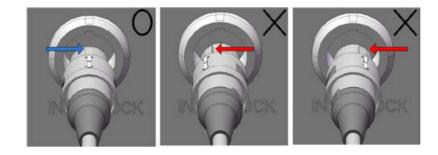
**IMPORTANT!** To connect or disconnect the sensor connector to the Neon<sup>™</sup> device, always handle the sensor connector using the cord plug and not the cord cable.
