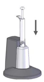
Note: Ensure the metal head of the Neon<sup>™</sup> Pipette is tightly connected to the ball plunger inside of the Neon<sup>™</sup> Pipette Station and to the Neon<sup>™</sup> Tube (see figure on the left for the correct position).
