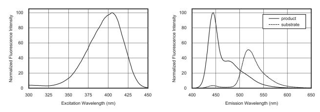
**Figure 2—Fluorescence excitation and emission spectra of LyticBLAzer**<sup>TM</sup>**\_h-FRET B/G.** The peak excitation wavelength for LyticBLAzer<sup>TM</sup>\_h-FRET B/G is 405 nm and the peak emission wavelengths are 445 nm and 520 nm.
