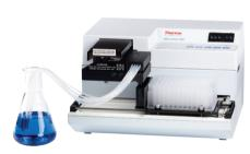
Multidrop DW dispenser is specially designed for dispensing into DW plates.
