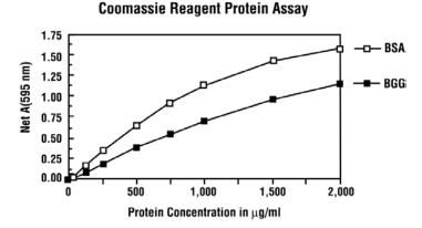
**Figure 1.** Typical color response curves for BSA and BGG using the Standard Test Tube Protocol of the Coomassie Assay.
