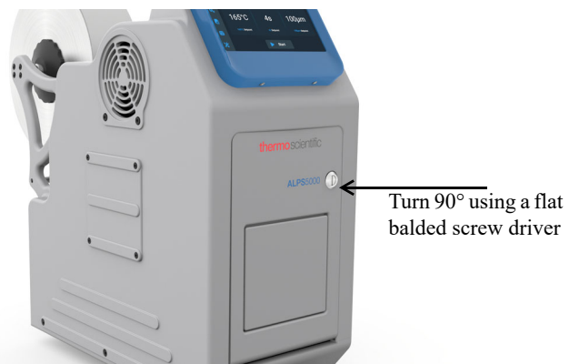
Figure 38. Unlock front service panel
