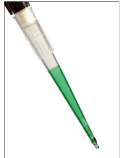
Conventional tip after dispensing 100 µL sample
