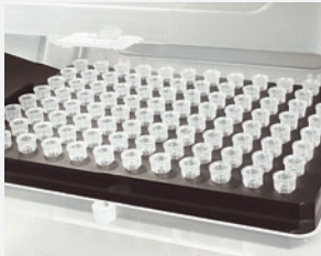
Axygen GEN3 10 \mu L multi-barrier tips, Maxymum Recovery surface
