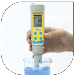
Step 1: Immerse tester sensor in solution
