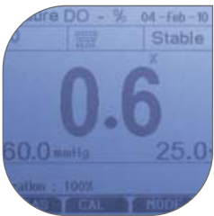
Stability display – faded out and then turns completely black when stable
