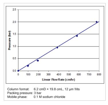
Figure 1 Pressure-flow properties of POROS™ XS resin
