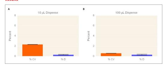
Figure 1. Analysis of EV-100-R tip with aqueous dispense. The precision (assessed by % CV) and accuracy (assessed by % D) of Axygen EV-100-R tips dispensing (A) 10  $\mu$ L and (B) 100  $\mu$ L volumes using the MCA head on the Tecan Freedom EVO liquid handling workstation were determined using the Artel MVS® system. The % CV and % D were below 2.5% for 10  $\mu$ L and below 1.0% for 100  $\mu$ L dispenses, n = 288.
