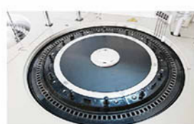
Reaction Tray 37±0.1°C, real-time monitor.
