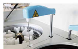
Sample Needle Liquid level sensor function. Anti-collision function. Reagent volume real-time detection.
