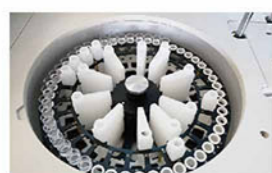
Reagent Tray 2~8°C cooling for 24 hours.
