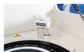
Washing Probe Independent 4-step washing system.
