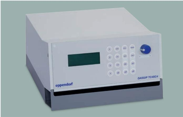
The DASGIP TC4SC4 provides four overhead drives with individual stirring speeds from 30 to 1,600 rpm, combined with precise temperature control. The TC4SC4D supports use of heat blankets, while the TC4SC4B can be operated with the DASGIP Bioblock. The Bioblock is an integrated solution for individual heating and cooling control of up to four bioreactors.
