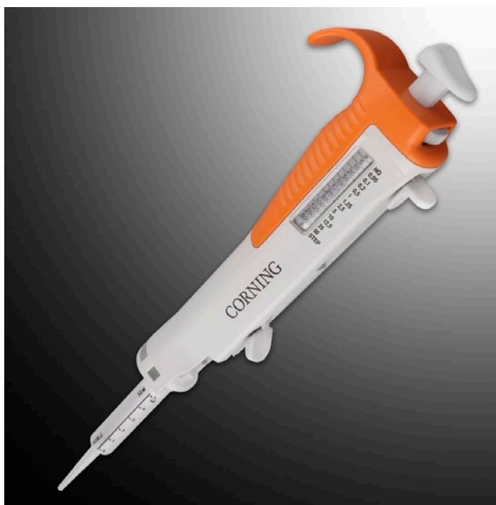
Corning Step-R is supplied with two syringe tip adapters (25 mL and 50 mL).
